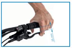
Try to move the bicycle while the brakes are activated. Both wheels must remain locked.
