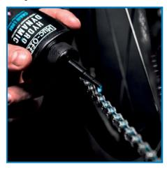
A chain with too much oil will accumulate more dirt and could get the other bicycle components, such as the brake pads, dirty and even damage them.
