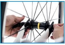
If the bicycle is not equipped with quick latches, the wheel must be fastened by tightening both sides of the nut/bolt system in a clockwise direction.
