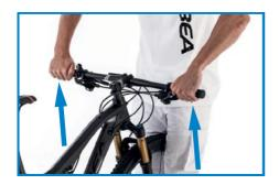
If the suspension fork shows any clearance, does not slide well or has any other anomaly, see an ORBEA dealer.
