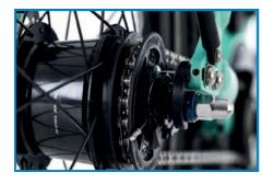
In both cases, it is important to make sure that the wheel axle is well seated on the frame before attaching the wheel and that the latches are completely closed, since they are responsible for fastening the wheel to the frame and the fork...
