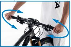
Mounting of the handlebar on the stem: (Frequency: Twice a year) To do this, hold the front wheel between your legs, grasp the handlebar on both ends and try to turn the handlebar on their own axis in both directions, making sure that the handlebar do not turn with respect to the stem, and that you do not hear any sort of noise or clicking sounds as you do it.
