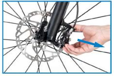
Jackets, cables and their tightening mechanism: (Frequency: Twice a year) The brake cables and jackets must not be scratched, bent, cut or worn. The brake cables must be fastened in the groove provided for this purpose and completely surrounding the cable.
