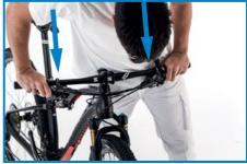
Clearance: (Frequency: Once a month) Holding the front wheel between your legs and try to lift the bicycle by the handlebar. The vertical bars must not move or come loose (apart from the contraction and expansion movement) from the insert bars or the fork plate.
