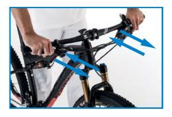
Excessive tightening: (Frequency: Twice a year) To check that the headset is not fastened too tight, suspend the bicycle so that the rear wheel is higher than the front one. Move the handlebar back and forth and then release them to check that the rear wheel and the handlebar return to their initial position without providing any sort of resistance.
