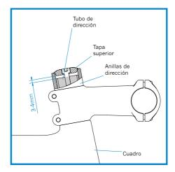
If more spacers are mounted under the stem to raise it and it extends more than 3-4 mm beyond the end of the head tube, it would be necessary to review the size of the frame or replace the stem with a model with a greater angle, under the supervision of an ORBEA dealer.
