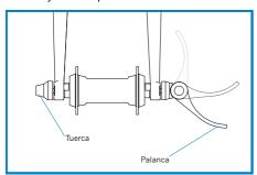
The quick latches have a nut on the opposite side of the lever. This nut may be a separate element or part of the frame/fork and it is used to give the initial tension to the system. To so this, before closing the lever that completely fastens the wheel, the shaft must be screwed in said nut, or vice versa. Screw it in until the lever can be closed with a certain amount of force (the force is considered
