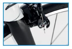
Correct mounting of the braking system: (Frequency: Twice a year) Check to see if they are mounted correctly, pulling by hand on the brake from in front of the front brake and from behind the rear brake.
