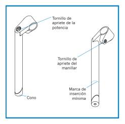
Loosen the tightening bolt, turning it twice in a counterclockwise direction.
