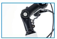
In the case that the stem has an angle adjustment bolt, the position of the handlebar can be adjusted more precisely; this can be done with the angle adjustment bolt.
