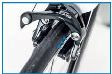
Symmetry between both brake shoes: (Twice a year)The brake shoes must have the same distance from the rim on both sides.
