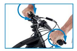
It is a good idea to also check that the components mounted on the handlebar, such as the brake levers, gear shits, jackets, horns or triathlon attachments are firmly fastened.
