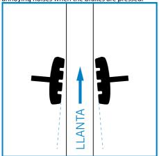
Brake shoe wear: (Frequency: Once a month) The brake shoes have grooves on them that must always be visible.
