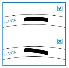
The brake shoes must not ever touch the tire, not even when the brake is not activated. If the brake shoes scrape the tire, this could tire, this could pop them as the result of wear or overheating.
