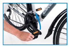
Regularly check that the reflectors on the pedals are clean and correctly positioned.
