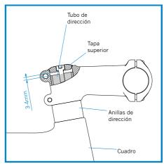
If all the spacers are below the stem, it must extend 3 to 4 mm above the end of the head tube.
