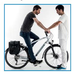
If when pedaling with great intensity, you notice an improvement when sliding back on the seat, it is likely that the seat is too low. If, on the other hand, the need is detected to move towards the tip of the seat to pedal, it is likely that the seat is too high.
