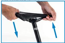
If the seat moves with respect to the seatpost, follow the instructions on the corresponding seatpost manual to attach it correctly.
