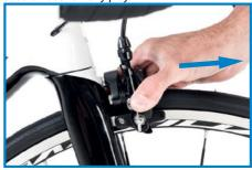
Position of the brake shoes: (Frequency: Every time the brake shoe is replaced) Brake shoes must be aligned in the center of the flank of the rim, approximately 1-2 mm from the top edge of the wheel.
