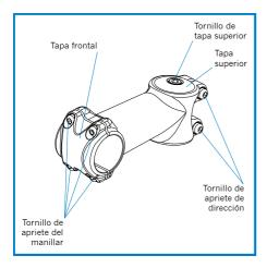
To invert the stem, separate the handlebar from the stem, removing the front cover from the stem.
